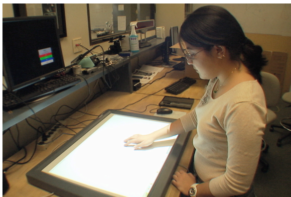
Figure 1. A user interacting with the MERL DiamondTouch screen. The DiamondTouch was evaluated in regards to task completion time and accuracy. A standard mouse was used for comparison.
